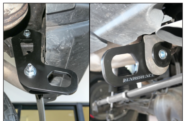
Illustration of installed state 安裝完成示意圖
