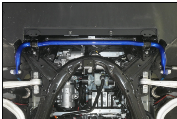
Illustration of installed state 安裝完成示意圖
