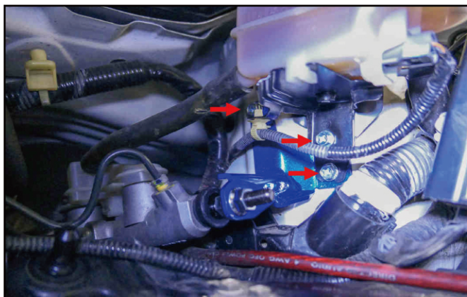
Illustration of installed state 安裝完成示意圖
