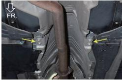
2. Attach ① Middle lower brace on to the vehicle. Once in place, reinstall the original bolts to secure the brace .(See figure 2) 將 ①中下結構桿 裝上車輛·完成後沿用原螺絲將拉桿鎖上車身。(請參照圖表二)
