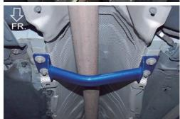
Illstration of installed state 完成示意圖
